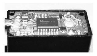
FIGURE 7.4 Hitec HS-311 electronics board.
