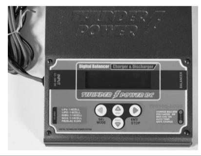
FIGURE 3.10 Automatic LiPo battery charger.
