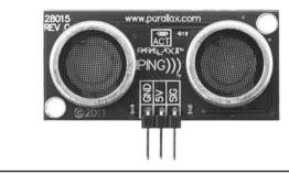
FIGURE 11.14 Parallax Ping sensor.
