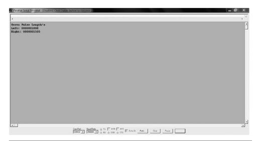
FIGURE 6.21 A Propeller Serial Terminal display of two servo channels.
