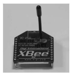
FIGURE 8.14 XBee Series 1 transceiver.
