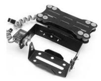
FIGURE 11.28 Pan-and-tilt mechanism for LIDAR mapping.
