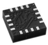
FIGURE 11.3 Honeywell three-axis compass sensor.
