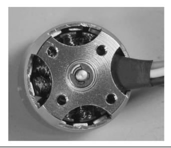
FIGURE 5.4 End view of the A2212/13T 1000KV motor.
