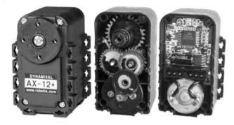
FIGURE 7.8 Dynamixel AS-12 digital servo interior views.
