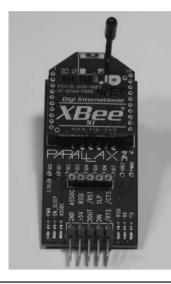
FIGURE 8.15 Parallax XBee SIP Adapter.
