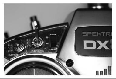
FIGURE 7.19 DX-8 Aux-1 (Flap) switch.
