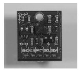
FIGURE 11.2 Parallax Compass Module HMC5883L.
