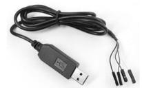
FIGURE 8.10 USB-to-TTL serial link cable.
