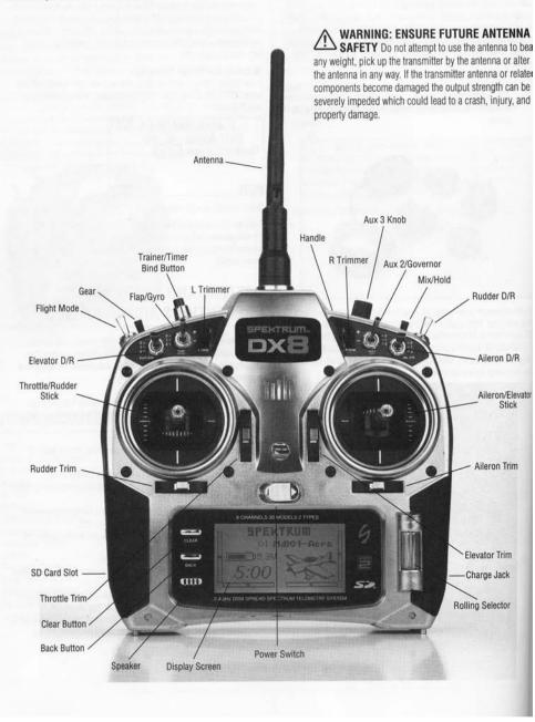
FIGURE 2.9 Spektrum DX-8 R/C transmitter.
