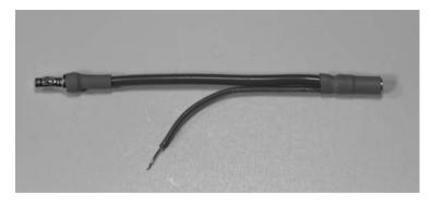
FIGURE 6.11 Test point extension cable.
