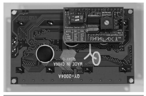
FIGURE 7.16 LCD display serial-to-parallel converter board.
