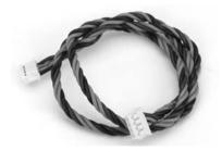
FIGURE 6.29 The X-BUS extension cable.
