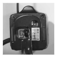
FIGURE 9.24 RC310 camera frequency selection switches.
