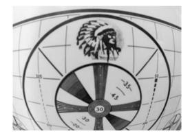
FIGURE 9.15 Hero 3 test-pattern image capture.
