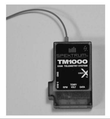
FIGURE 3.13 Spektrum 1000 telemetry transmitter.
