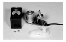
FIGURE 7.2 Disassembled servo showing the feedback potentiometer.
