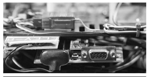
FIGURE 7.18 Early version of an Elev-8 LED-lighting controller.
