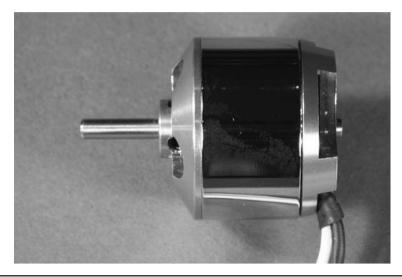
FIGURE 5.1 Elev-8 BLDC motor A2212/13T 1000KV.
