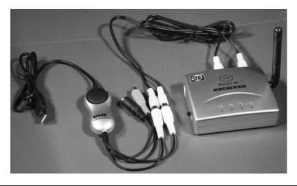
FIGURE 9.23 RC310 receiver and an EzCap USB video-capture module.
