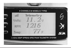
FIGURE 6.25 The DX-8 LCD showing real-time telemetry.
