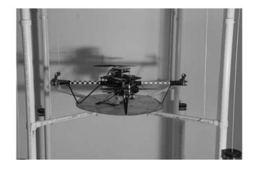
FIGURE 10.19 The Elev-8 mounted on the test frame.
