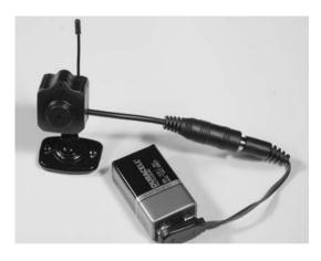
FIGURE 9.20 The RC310 camera-transmitter module.
