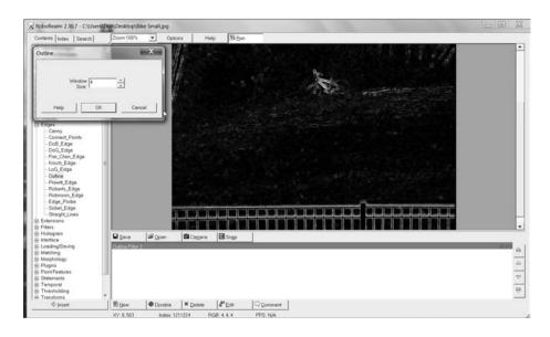
FIGURE 9.43 Outline edge detection of the high-resolution test image.
